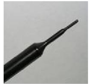
Figure 4.4 EX3DV4 E-field Probe
