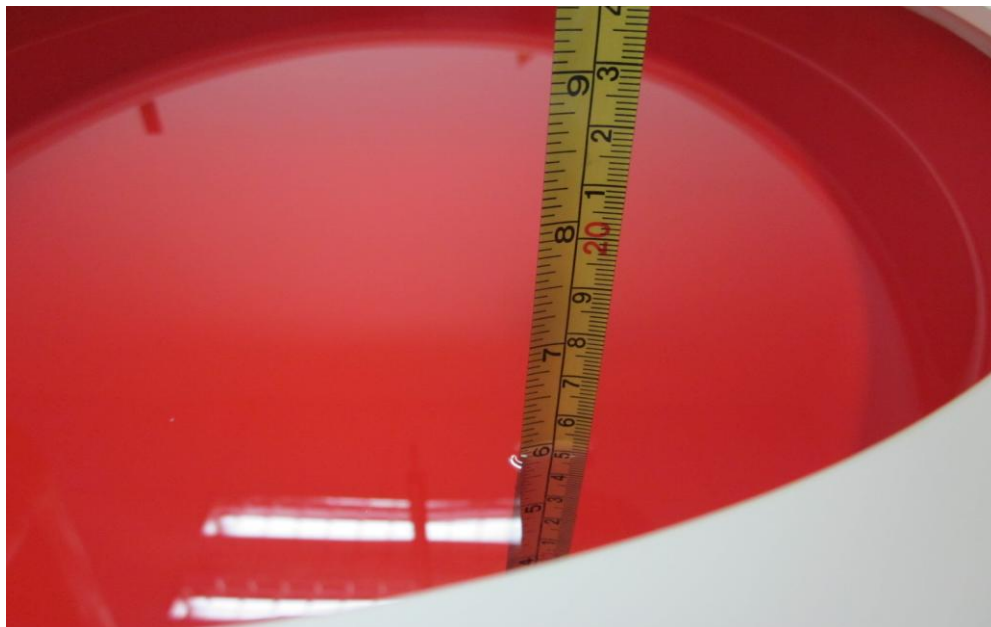
Figure 4.4: Liquid depth in the Flat Phantom
