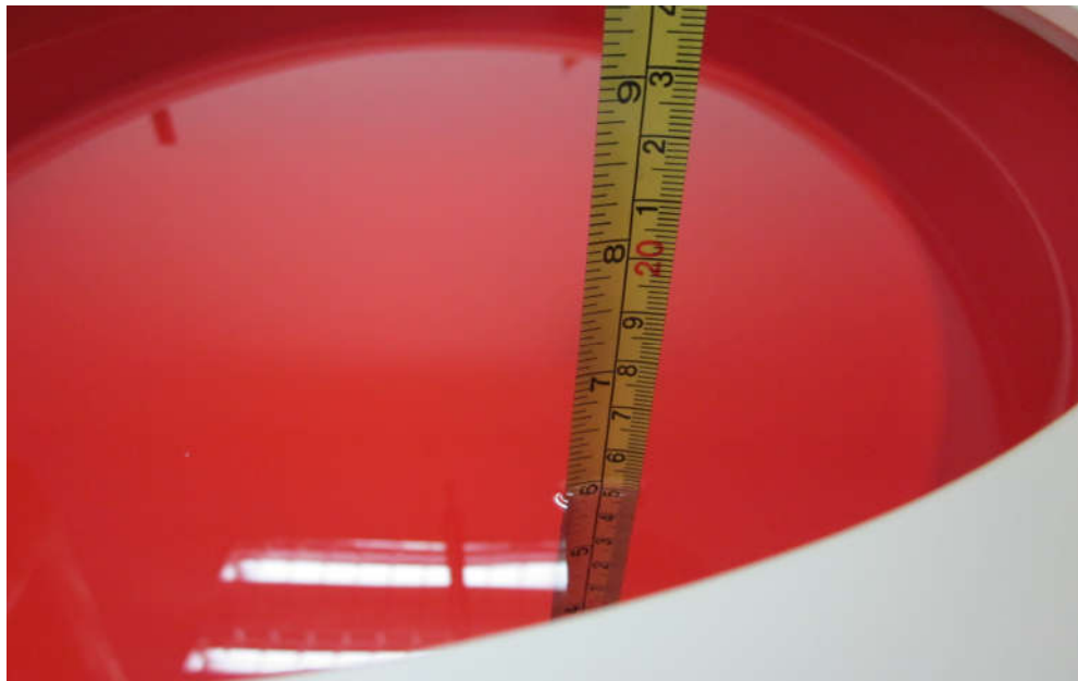
Figure 4.4: Liquid depth in the Flat Phantom
