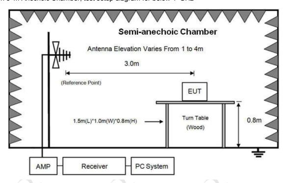
Semi-Anechoic 3m Chamber
