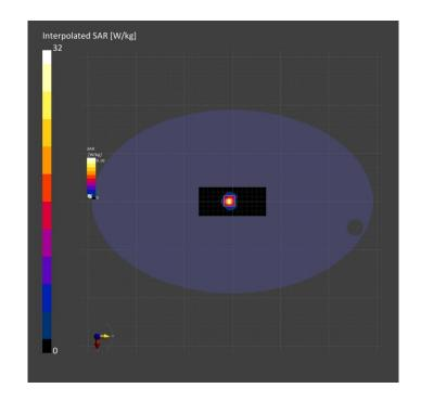
Measurement Report for Device, FRONT, D5GHz, UID 0 -, Channel 60 (5600.0MHz)
