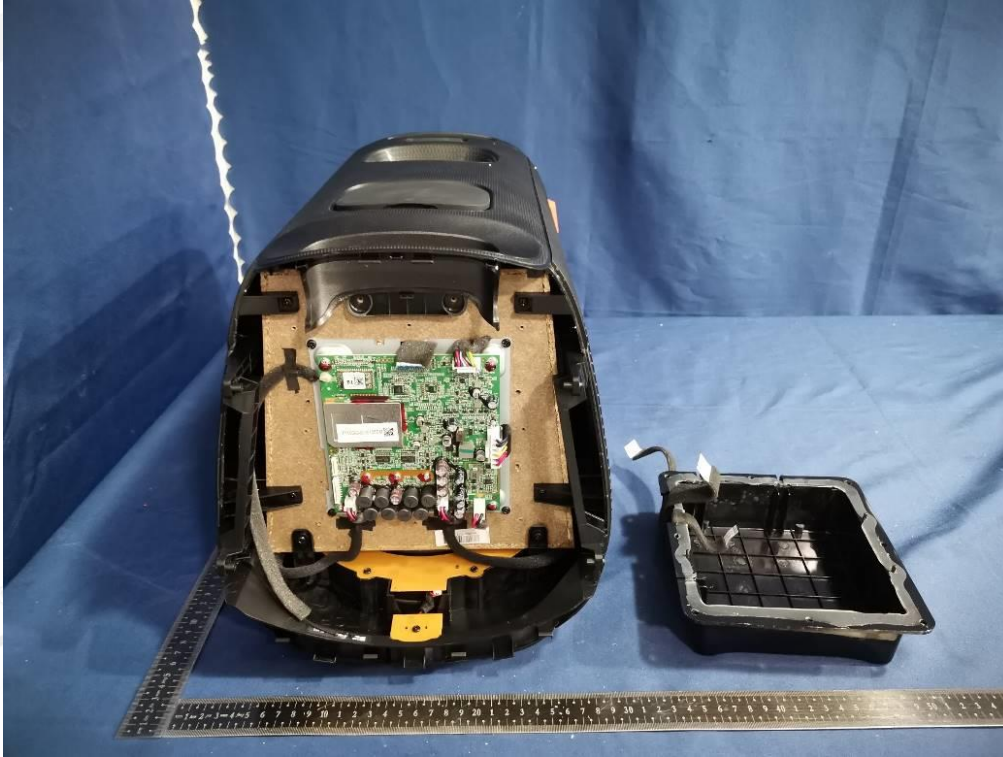
Mainboard B + AY power board + Battery(IDA108GA)
