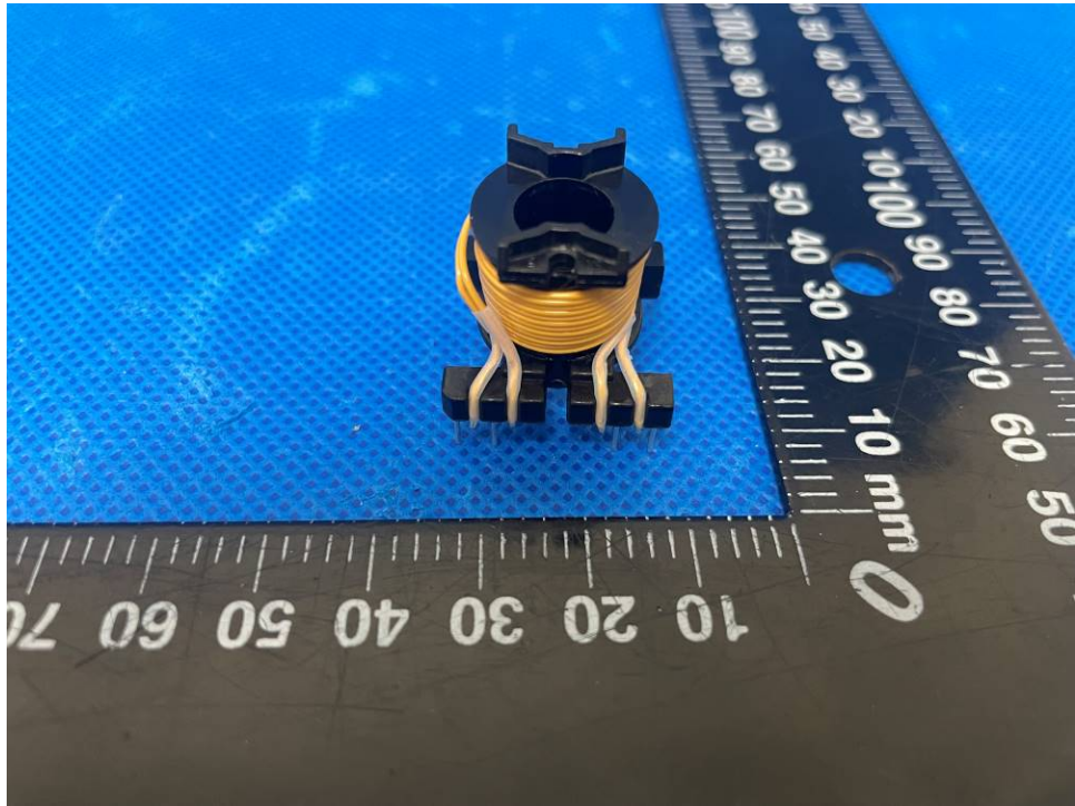
Figure 39. Transformer T901 view 11
