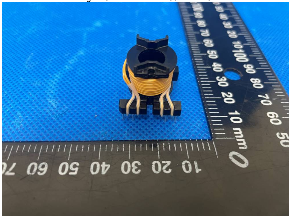
Figure 38. Transformer T902 view 11
