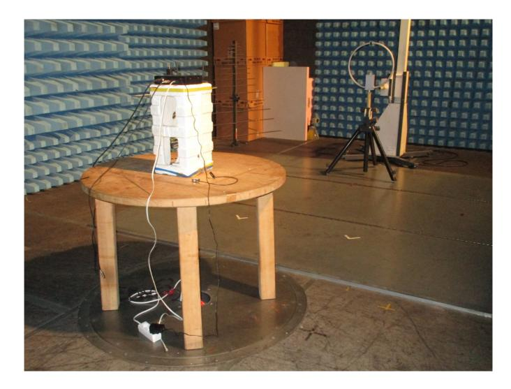
Description: Test setup 30 MHz - 1 GHz
