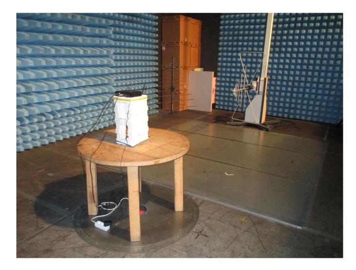
Description: Test setup above 1 GHz
