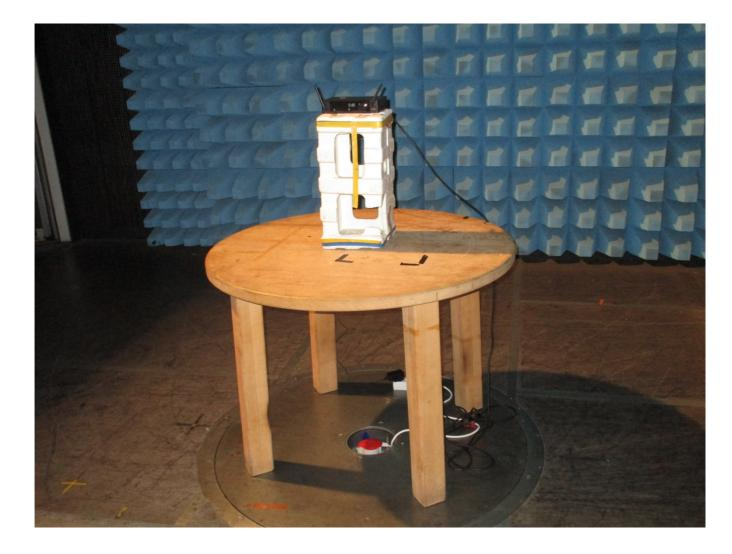
Description: Test setup up to 30 MHz
