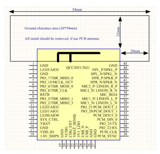
A. If there is battery, metal, LCD, loudspeaker, etc. beside the module antenna, it is required to be at least 15mm away from the antenna
