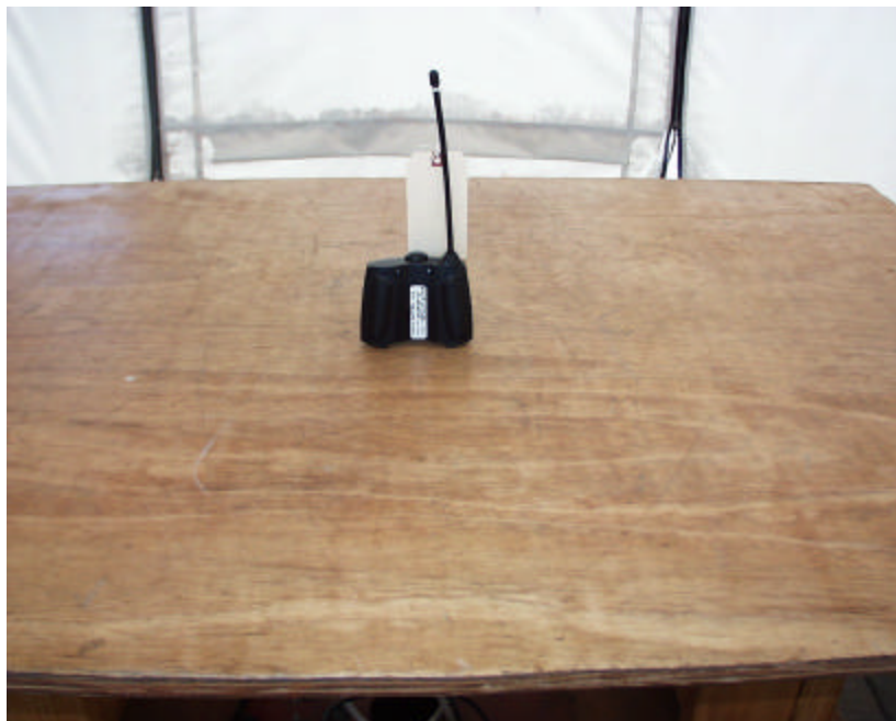
Radiated Open Site Test Set-up
