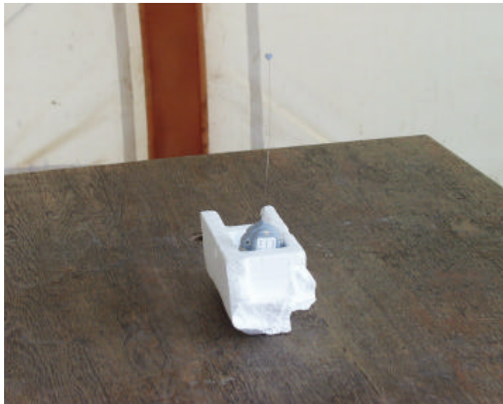
Radiated Open Site Test Set-up
