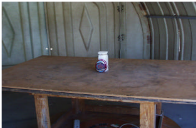
Radiated Open Site Test Set-up
