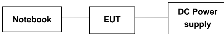
Fig. 2-1 Configuration of Conducted & Radiated Emission Tested System n
