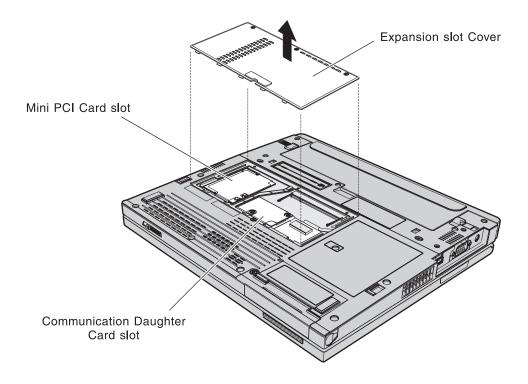
**Attention:** The ThinkPad X41 Tablet Series computer contains an authentication mechanism If you install an unauthorized wireless LAN Mini-PCI Card or RF CDC module that is not approved for use in the ThinkPad X41 Tablet Series computer, the computer will not start, but only displays an error message and emits beeps.
