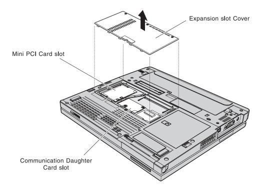
**Attention:** The ThinkPad X41 Tablet Series computer contains an authentication mechanism You can install or remove each wireless feature by yourself. If you install an unauthorized wireless adapter that is not approved for use in the ThinkPad X41 Tablet Series computer, the computer will not start, but only displays an error message and emits beeps.
