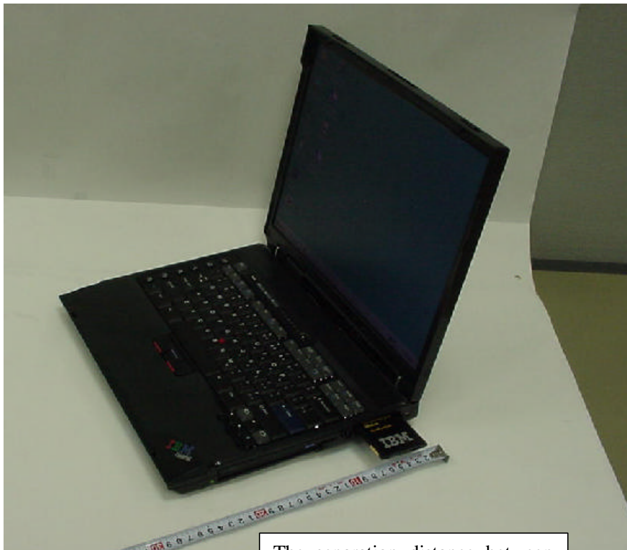
The separation distance between the antenna and the human body is longer than 20cm.
