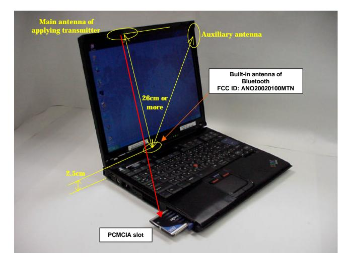
The main and auxiliary antennas located at LCD section of the host devices (ThinkPad T40 or R50 Series) are assembled apart from each Bluetooth antenna with 26 cm or more as shown in the previous page.
