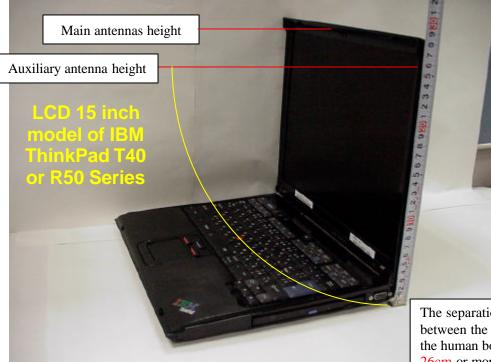
The separation distance between the antenna and the human body (lap) is 26cm or more.
