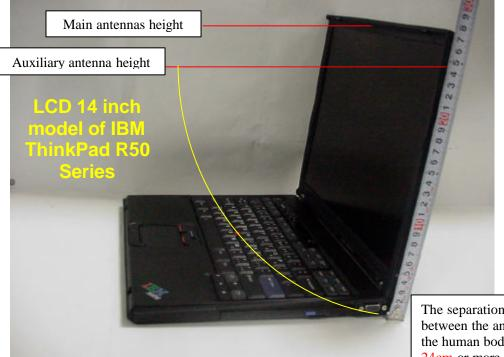
The separation distance between the antenna and the human body (lap) is 24cm or more.
