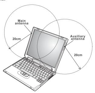
Note: IBM Dual-Band 11a/b Wi-Fi Wireless Mini PCI Adapter implements transmission diversity function. The function does not emit radio frequencies simultaneously from both antennas. One of the antennas is selected automatically or manually (by users) to have good quality of radiocommunication.
