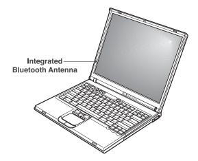
**Note:** The antenna of IBM Integrated Bluetooth with 56K Modem is located on the left side of the computer lid. Transmitted energy from the Bluetooth device is very low compared to other RF devices. Therefore a 20 cm separation from the Bluetooth antenna is not required.
