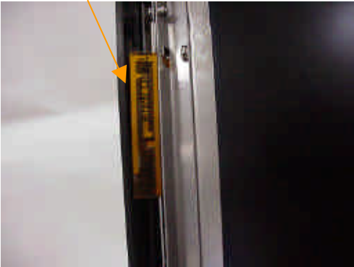
Main antenna Dual Band Inverted-F type P/N: 3301BZ9076A
