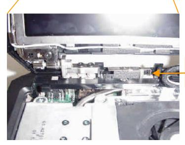
Auxiliary antenna Inverted-F type P/N: 46L6324
