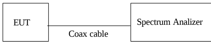
Figure 1: Measurement setup for 6dB bandwidth test
