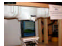
Figure A.4.4 Body SAR Test Setup -- Tablet Position, LCD Flip -- (Left Side)
