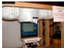
Figure A.8.1 Body SAR Test Setup -- Tablet Position, LCD Open -- (Top Side)
