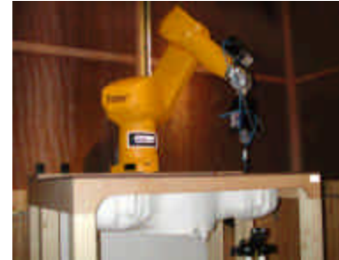
Figure 6.1 DASY4 Test System
