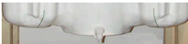
Figure 7.2 SAM Twin Phantom shell
