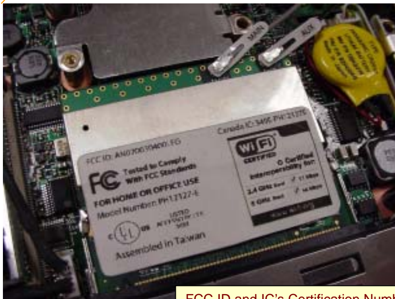
FCC ID and IC's Certification Number is visible when the keyboard assembly is removed.
