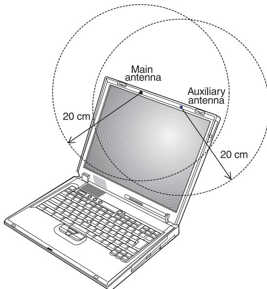
**Note** The IBM Dual-Band 11a/b Wi-Fi<sup>®</sup> Wireless Mini PCI Adapter implements transmission diversity function. The function does not emit radio frequencies simultaneously from both antennas. One of the antennas is selected automatically or manually (by users) to have good quality of radio communication.
