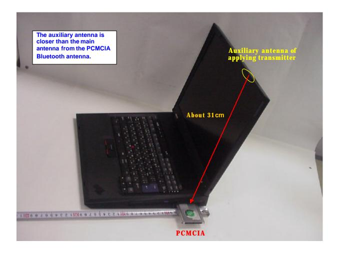
The main and auxiliary antennas of the applying transmitter in the LCD section are assembled apart from the Bluetooth antenna shown in the previous page with 20 cm or more distance.
