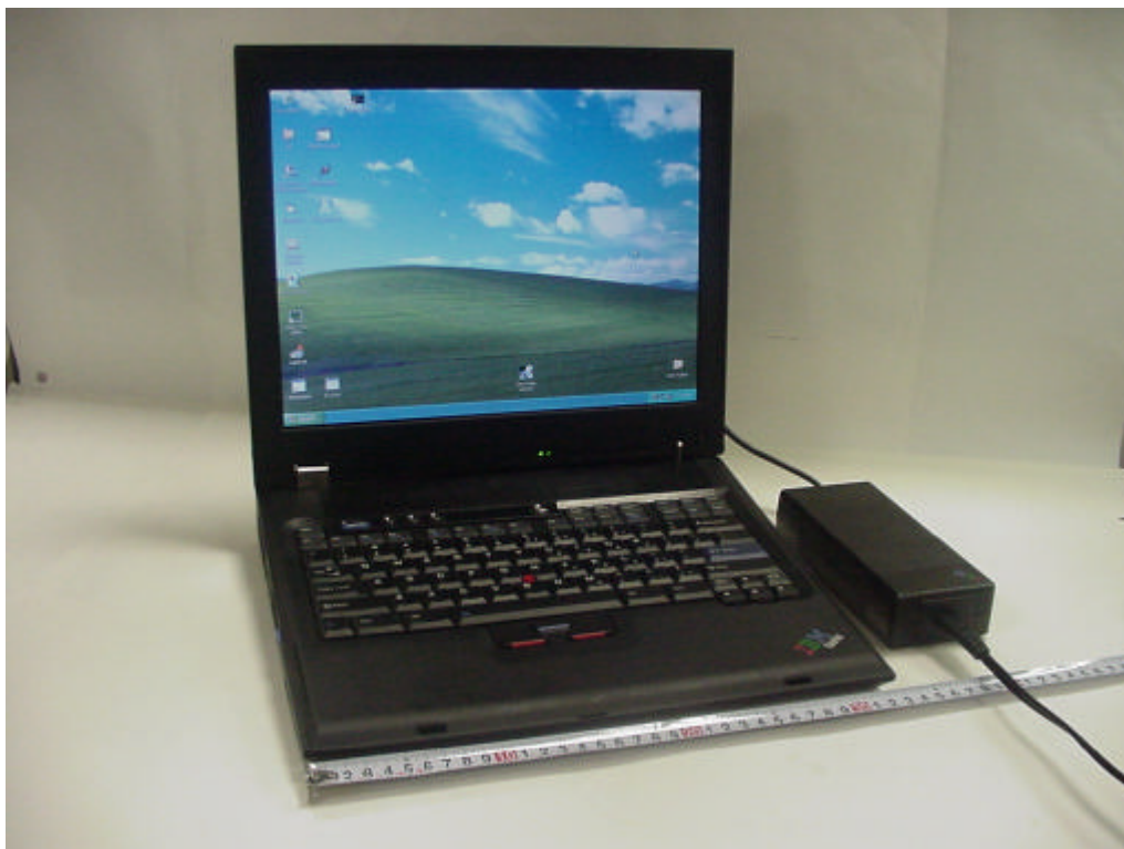
IBM ThinkPad G40 Series (LCD 14" Model), Front View
