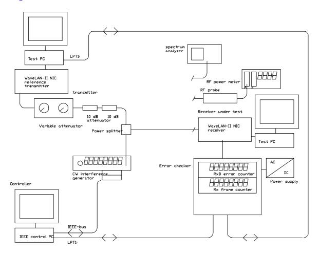
Figure 1, measurement test set-up.
