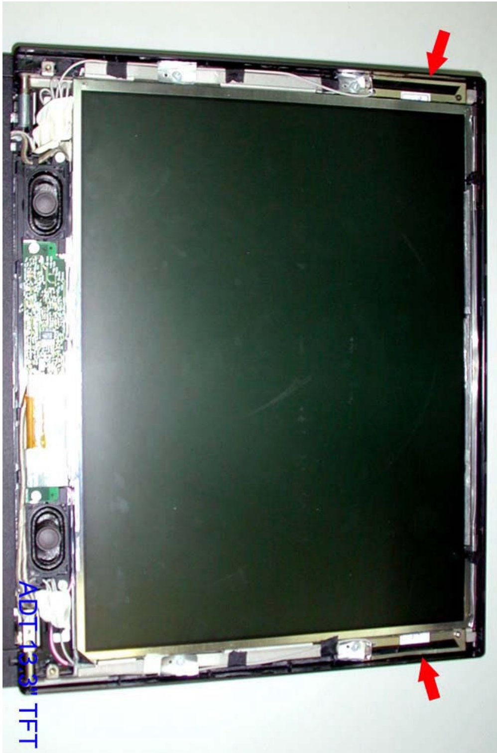
Photo.8: Diversity Antennas mounted in LCD IBM ThinkPad i Series 1300 (1171-71U, 13 inch LCD)
