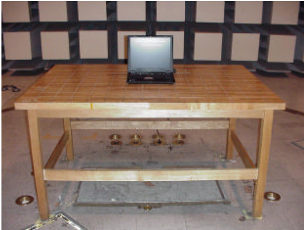
Radiated Emission - Front View (EMI SEMIANECHOIC CHAMBER)
