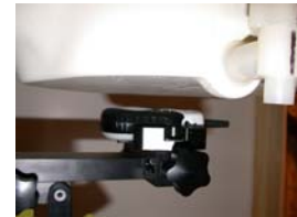
Figure 14.2 Face SAR Test Setup -- FRS --
