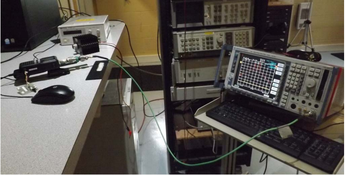
Figure E23.1 – Setup, Conducted Measurements
