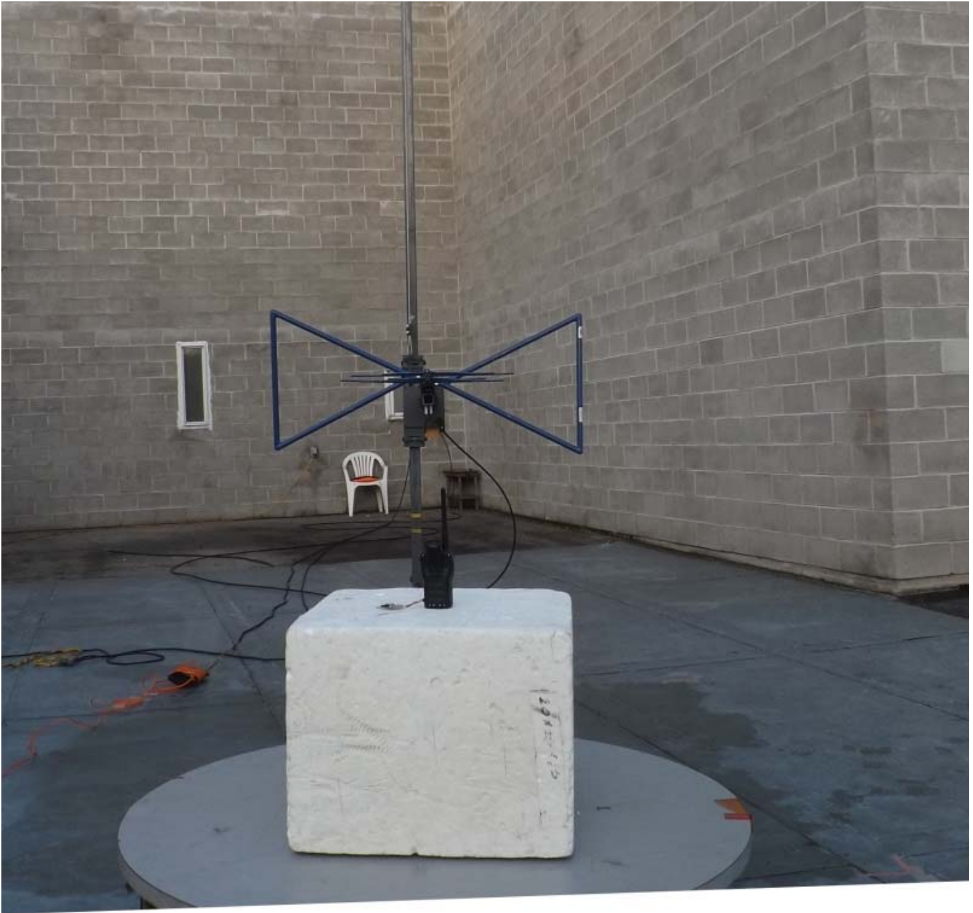
Figure E23.5 – Setup, Radiated Measurements Below 1GHz
