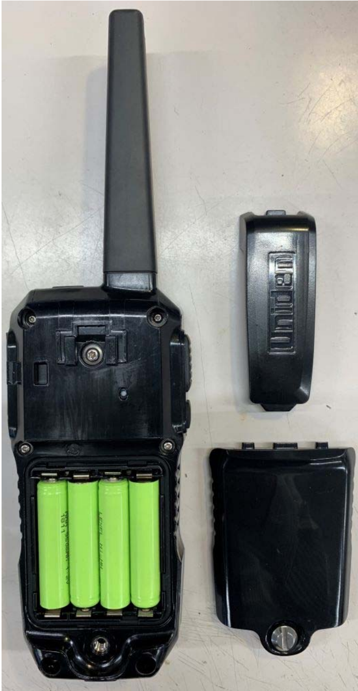
Figure E19.1 – Internal Photo – Battery Cover Removed
