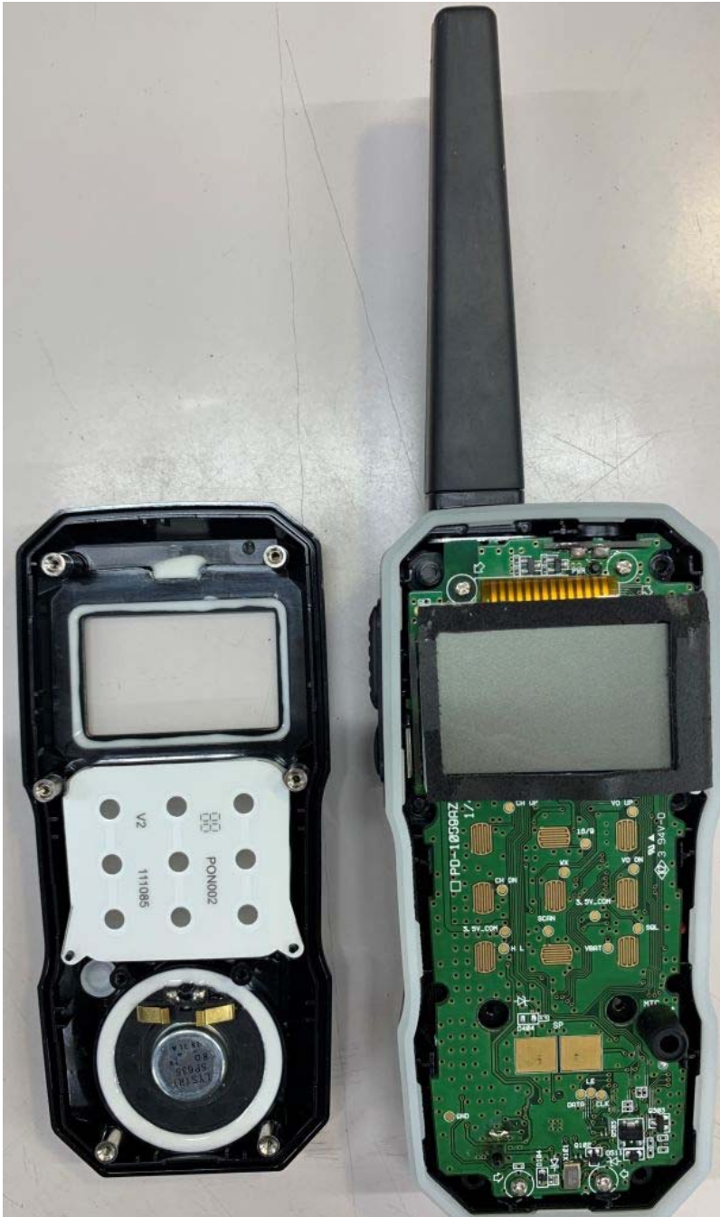
Figure E19.3 – Internal Photo – Front Cover Removed – Main PCB Display Side
