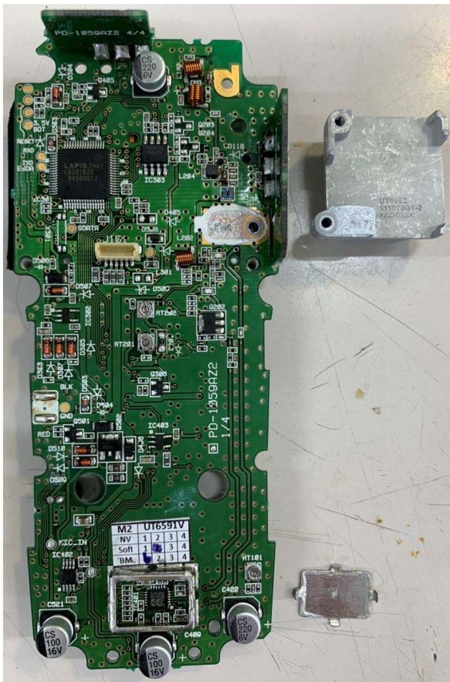
Figure E19.6 – Internal Photo – Main PCB Component Side – Heat Sinks Removed
