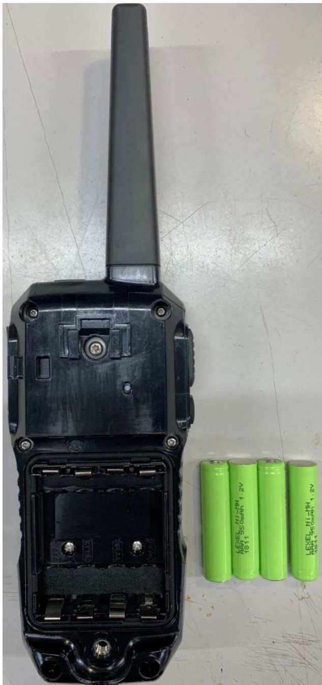
Figure E19.2 – Internal Photo – Batteries Removed
