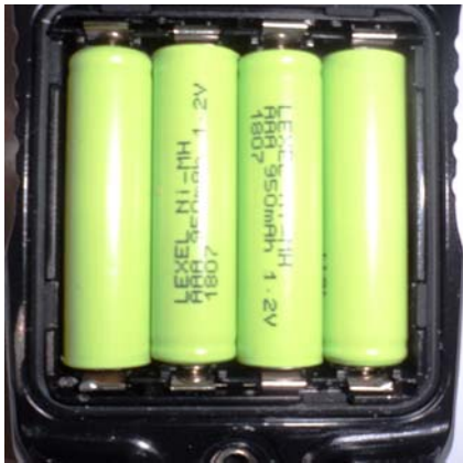
P1 Battery Pack (AAA 1.2V) NiMH Rechargeable
