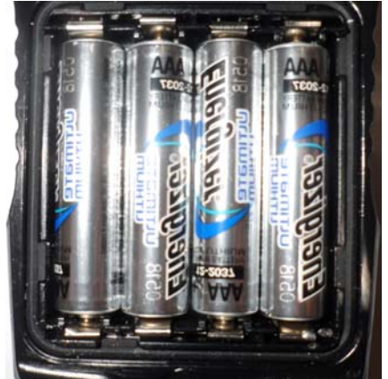
P3 Battery Pack (AAA 1.5V) Li-Ion Non Rechargeable
