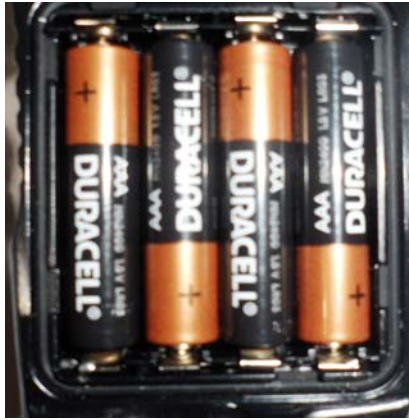
P2 Battery Pack (AAA 1.5V) Alkaline Non Rechargeable
