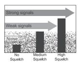
While listening to a channel, adjust the **SQUELCH** knob until the noise is filtered out and you can only hear the transmission. If you switch to a channel with a lot of noise or with a weak transmission, you may need to adjust the squelch level again.
