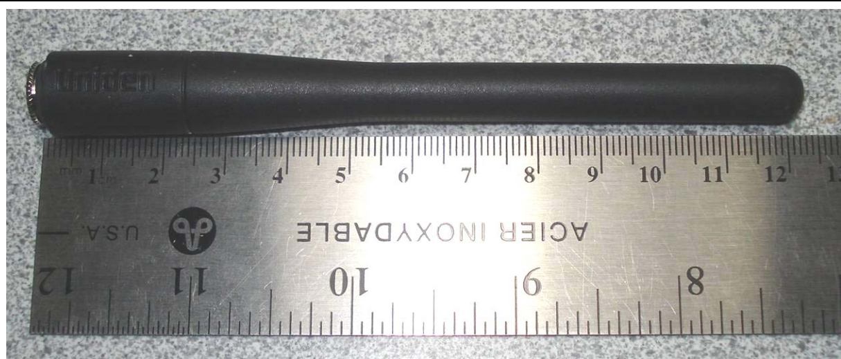
Flexible Whip Antenna (P/N: BATG0565001)
