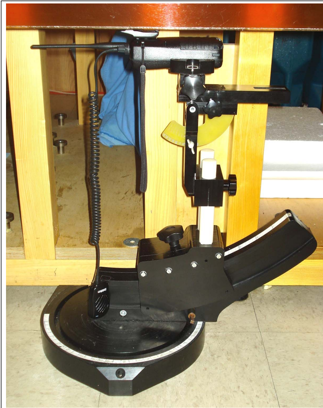
Body-worn Configuration - DUT with Belt-Clip Accessory & Speaker-Microphone Audio Accessory (P/N: 12012597)
