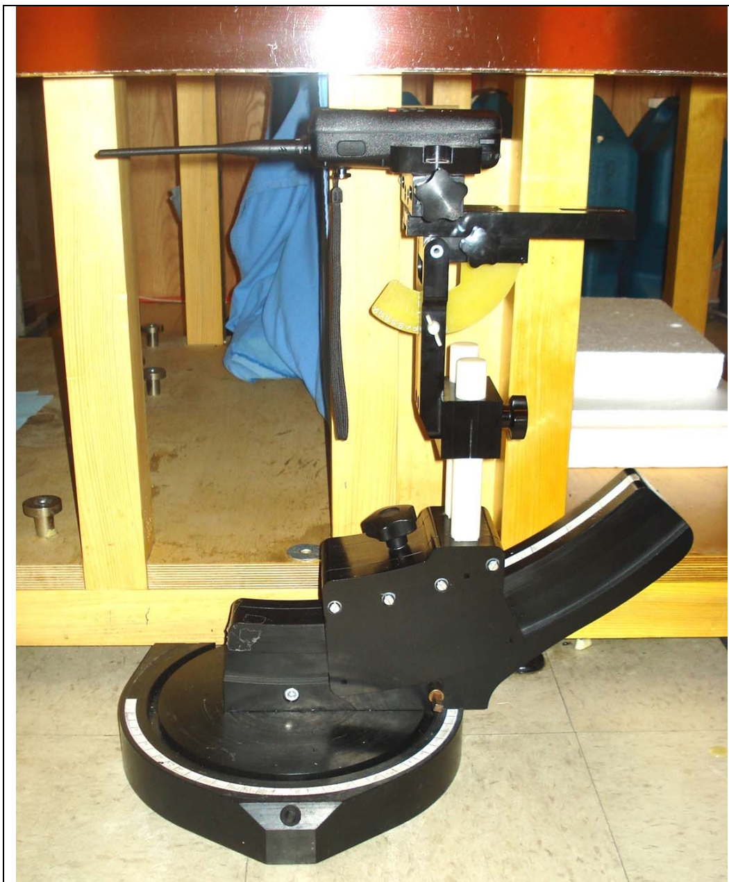
Face-held Configuration - DUT with 2.5 cm spacing from front keypad side of radio to planar phantom
