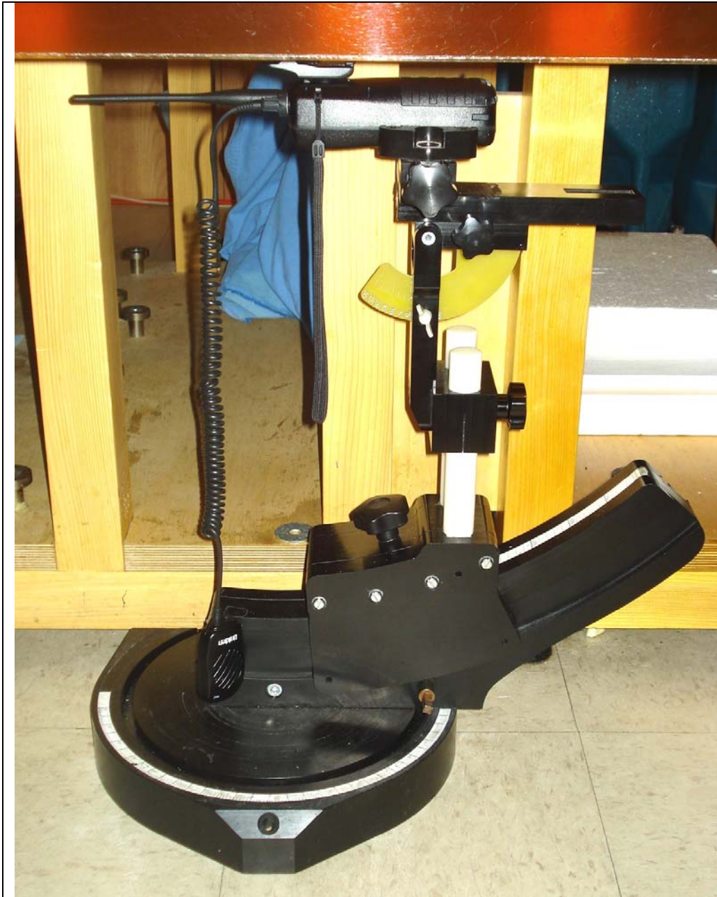
Body-worn Configuration - DUT with Belt-Clip Accessory & Speaker-Microphone Audio Accessory (P/N: 12012597)
