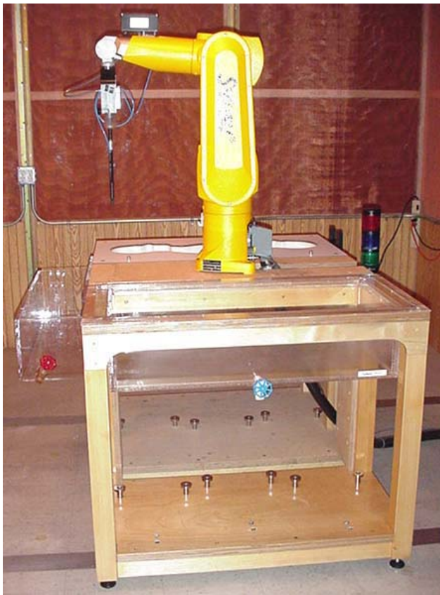
DASY4 SAR Measurement System with validation phantom
