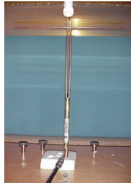
300MHz Dipole Setup
