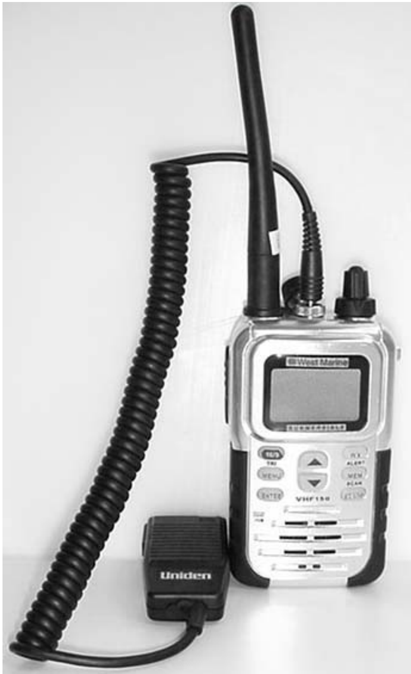
DUT with Speaker-Microphone Audio Accessory (Model: HHVTA07)
