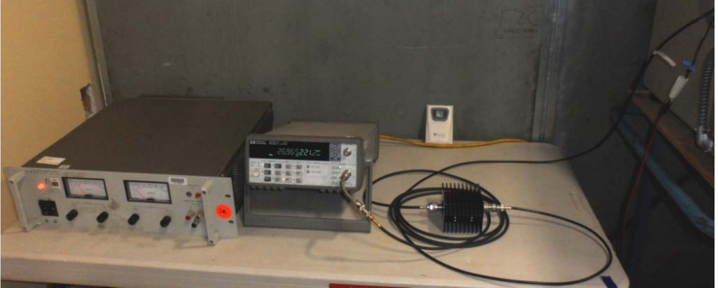
Figure E21.4 – Setup Photo – Frequency Stability Measurements
