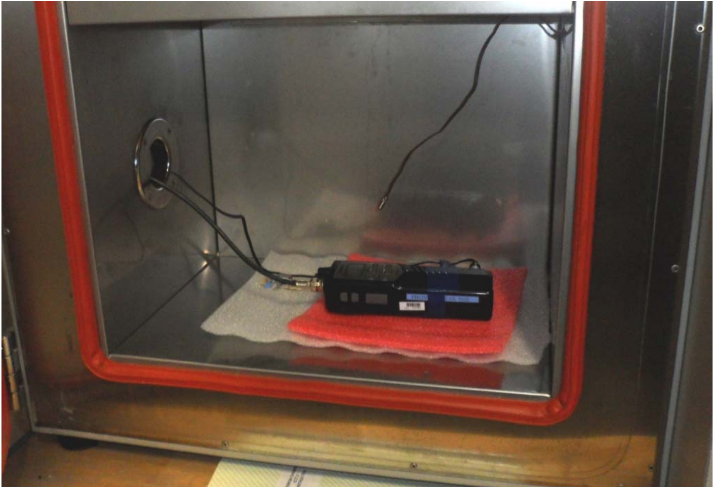
Figure E21.5 – Setup Photo – Frequency Stability Measurements
