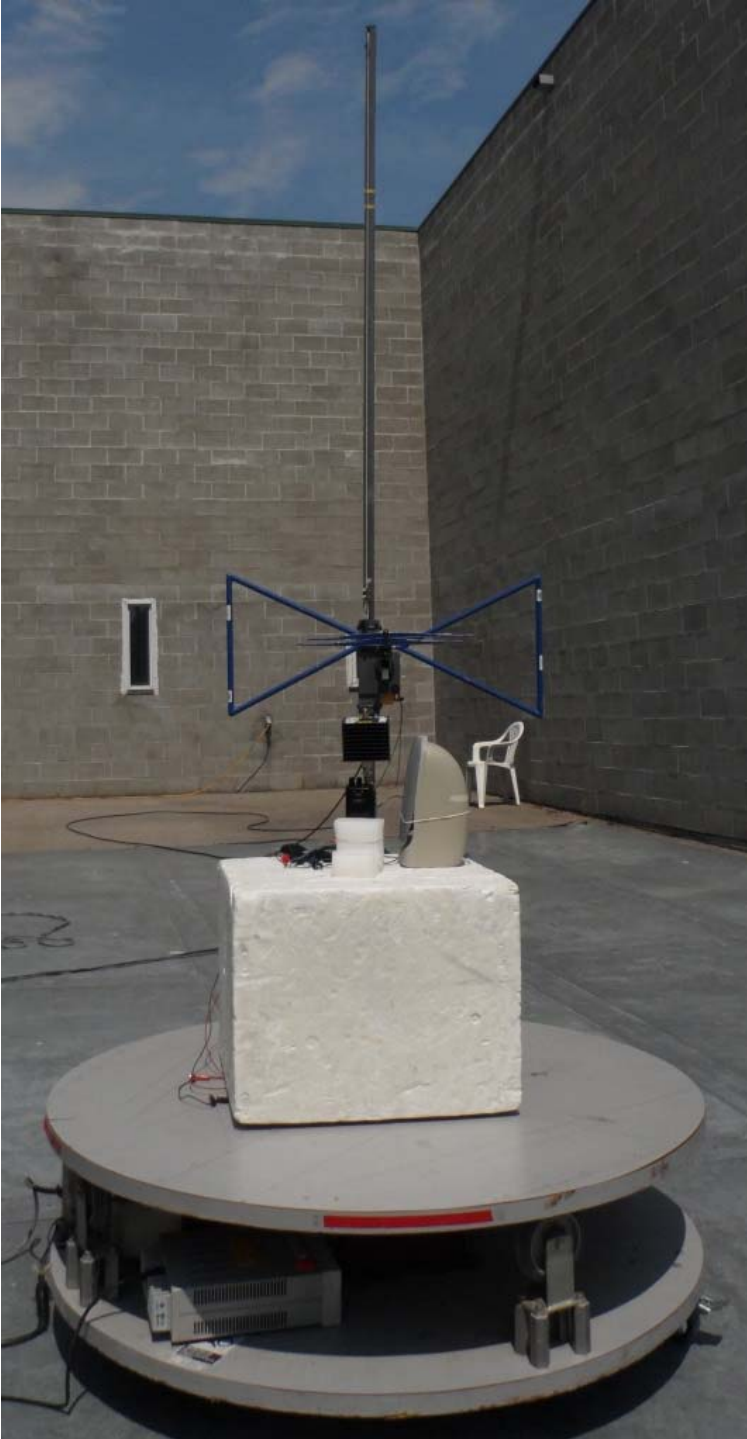
Figure E21.6 – Setup Photo – Radiated Measurements - Horizontal
