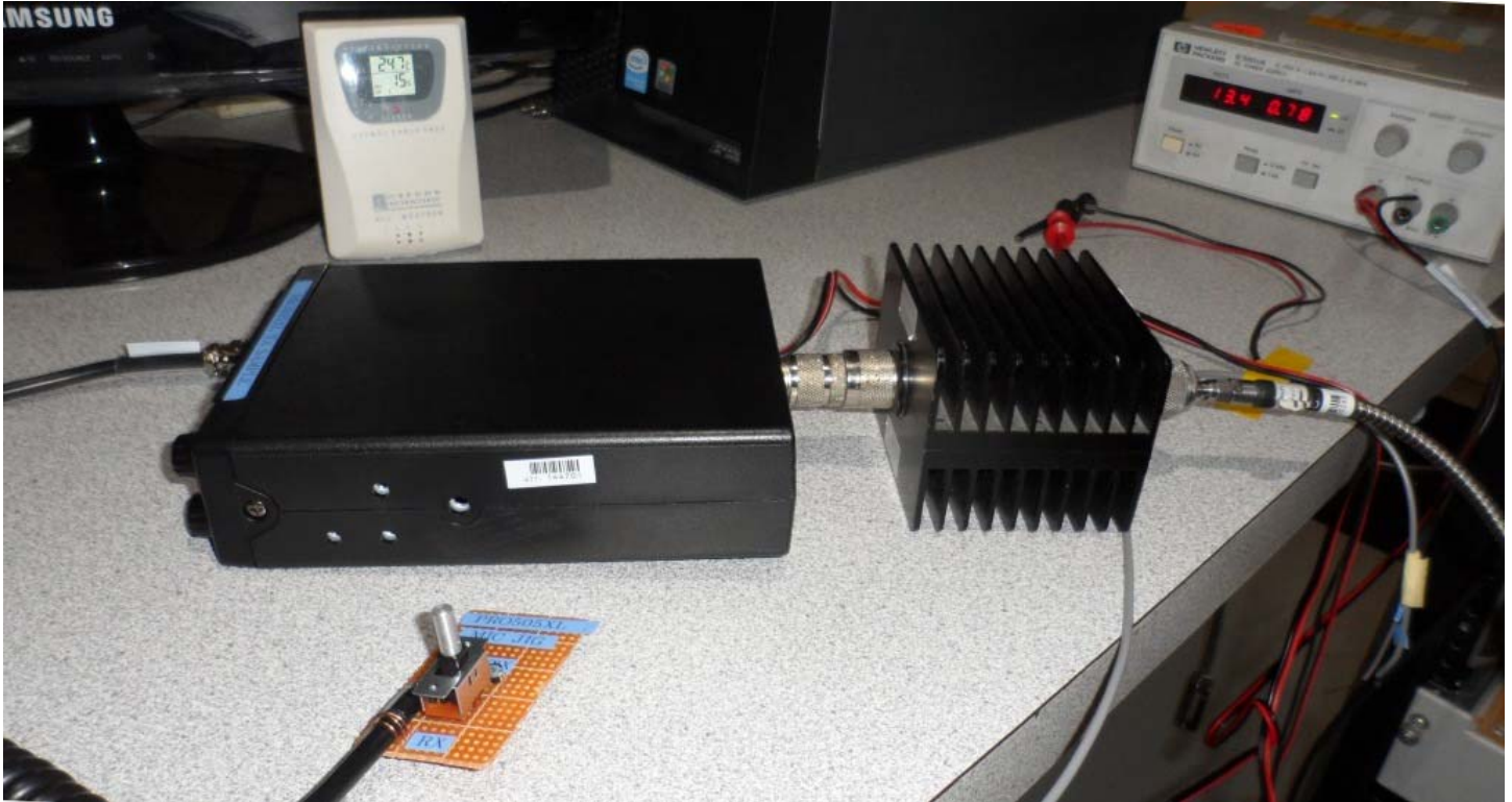
Figure E21.1 – Setup Photo – Conducted Measurements
