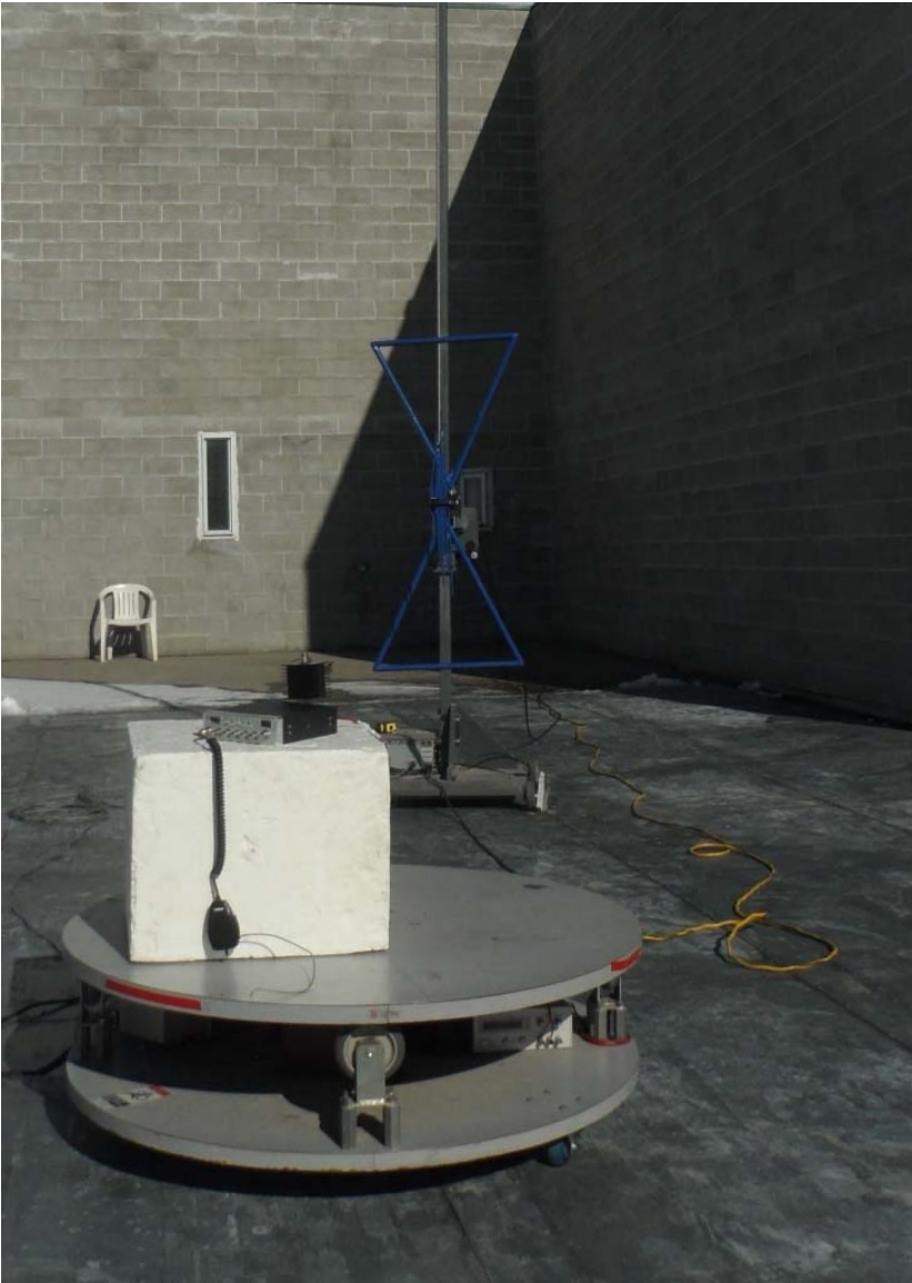
Figure E14.3 – Setup Photo – Radiated Emissions < 1GHz
