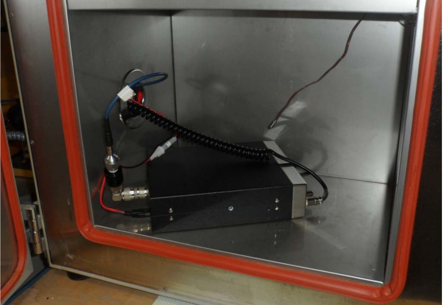
Figure E14.1 – Setup Photo – Frequency Stability – DUT in Environmental Chamber
