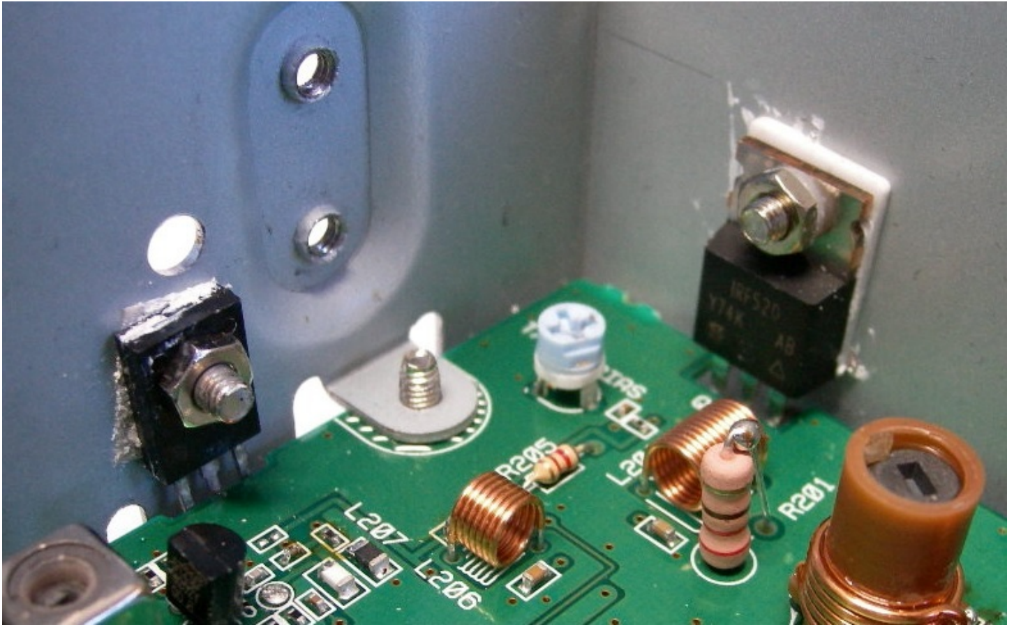
Figure E13.10 – Internal Photo – PCB – RF Amplifier Section
