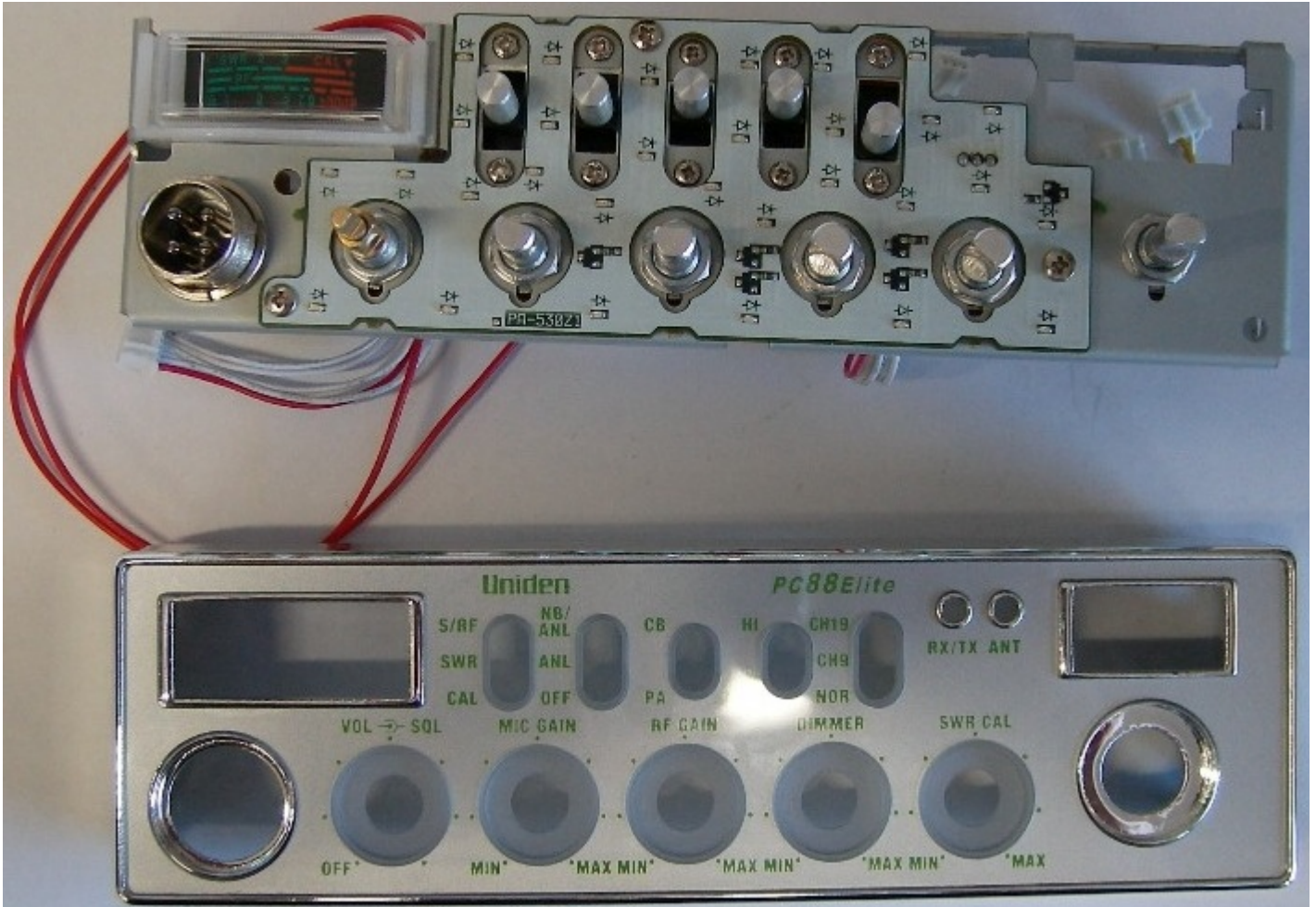
Figure E13.4 – Internal Photo – Front Control Assembly – Front View
