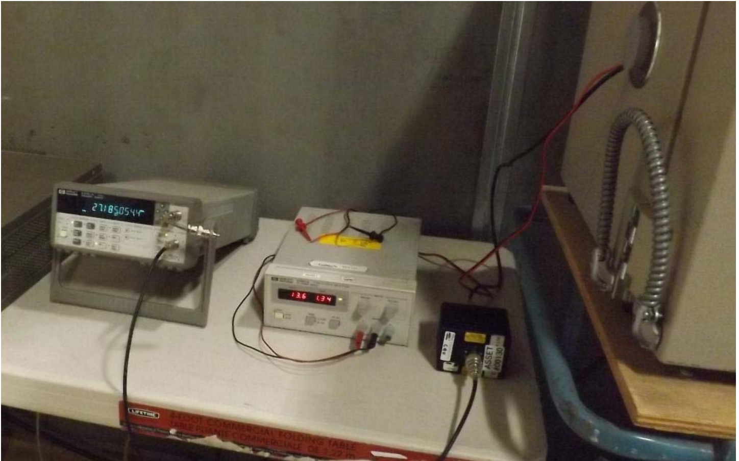
Figure E23.8 – Setup, Frequency Stability
