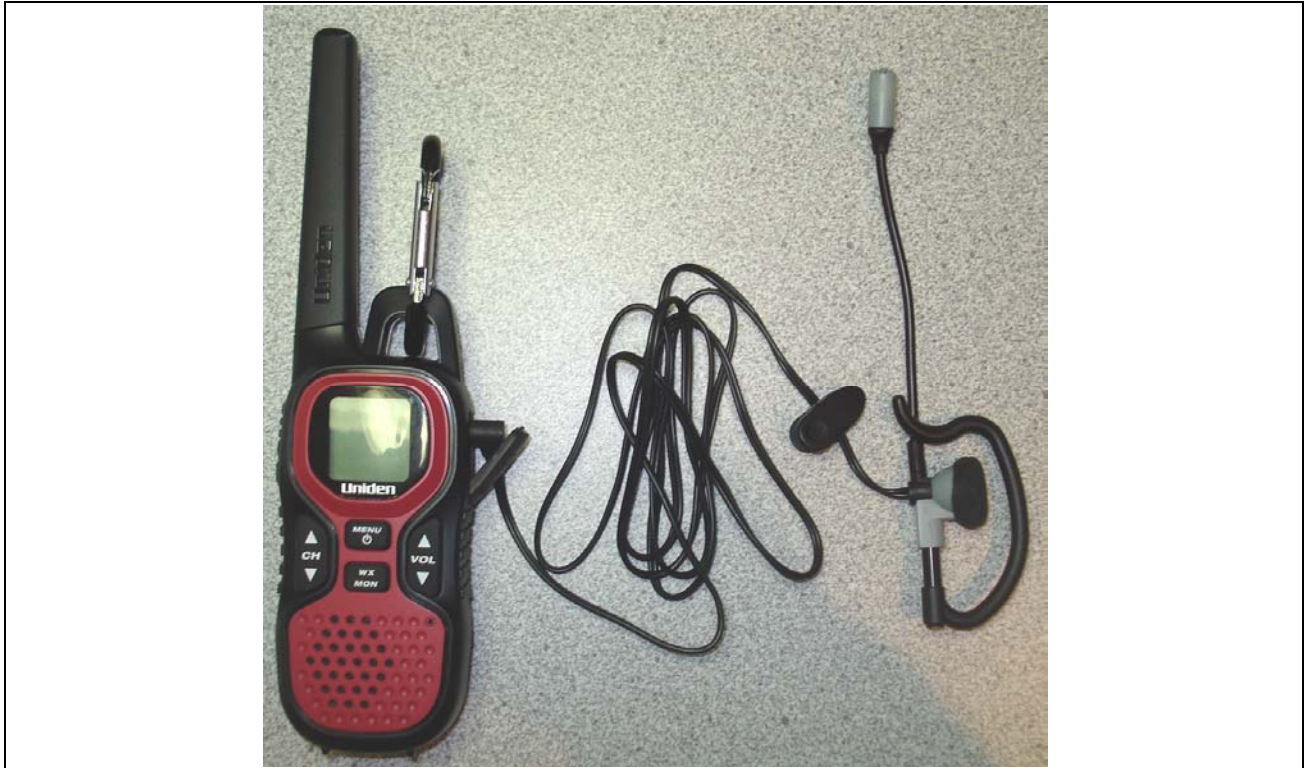
Front of DUT with Carabiner and Headset/Boom-Microphone audio accessory (P/N: ZA-133)
