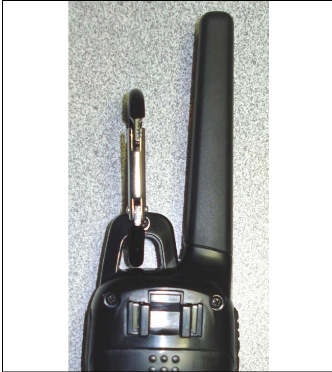
Back of DUT with Carabiner body-worn accessory
