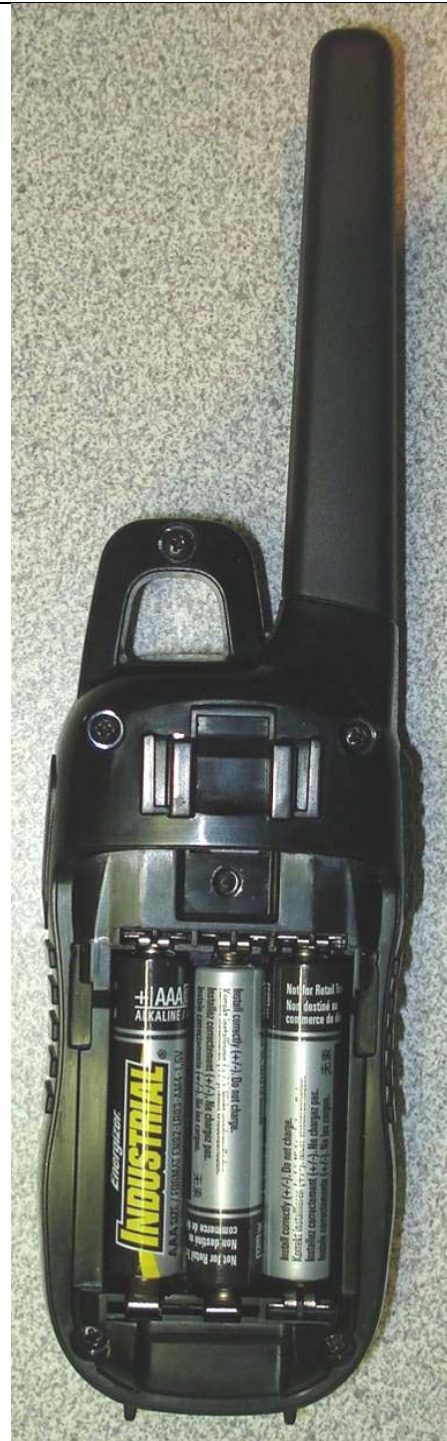
Back of DUT with Alkaline batteries
