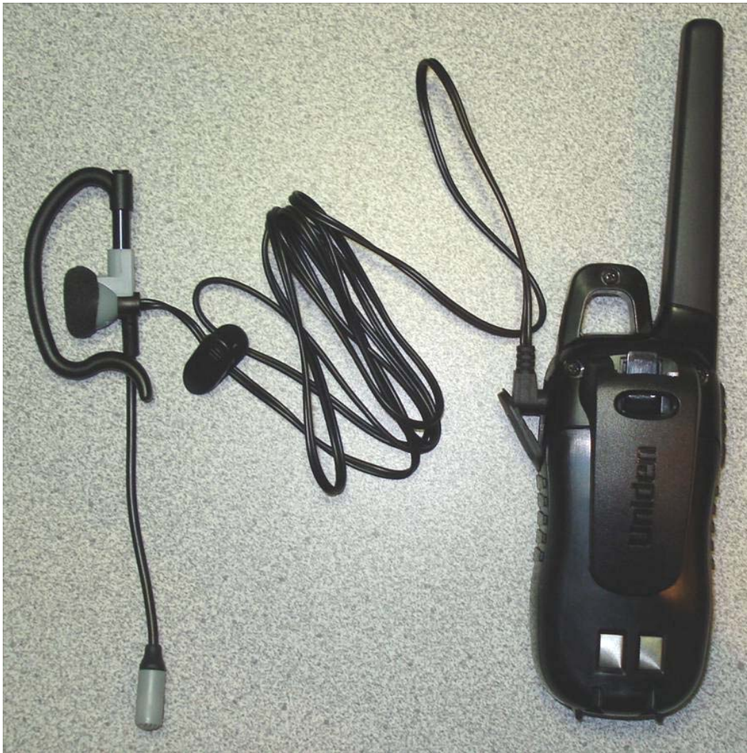
Back of DUT with Plastic Belt-clip and Headset/Boom-Microphone audio accessory (P/N: ZA-133)
