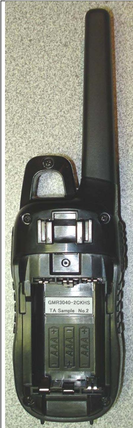
Back of DUT with battery cover removed
