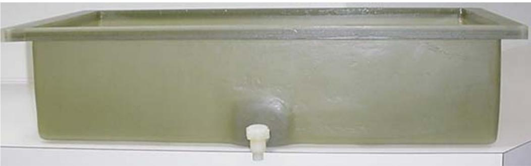
**Fiberglass Planar Phantom - Front View**
