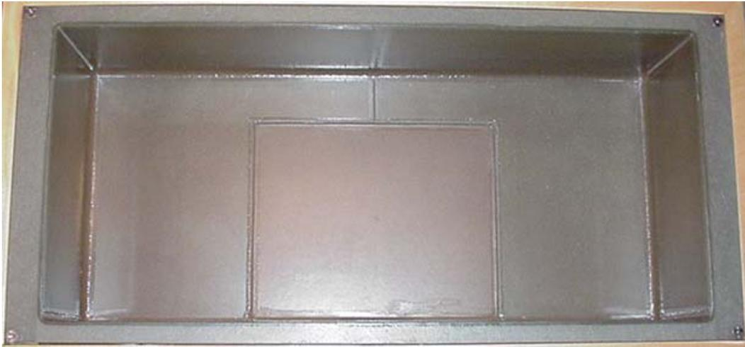
**Fiberglass Planar Phantom - Top View**
