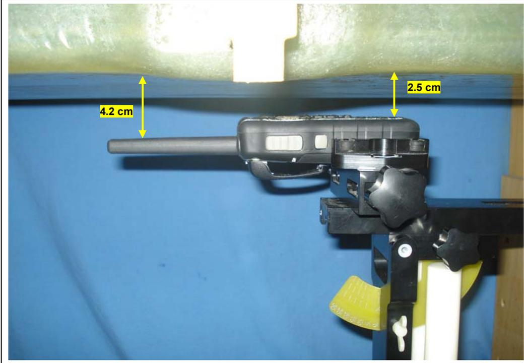
**BODY-WORN SAR TEST SETUP PHOTOGRAPHS**
