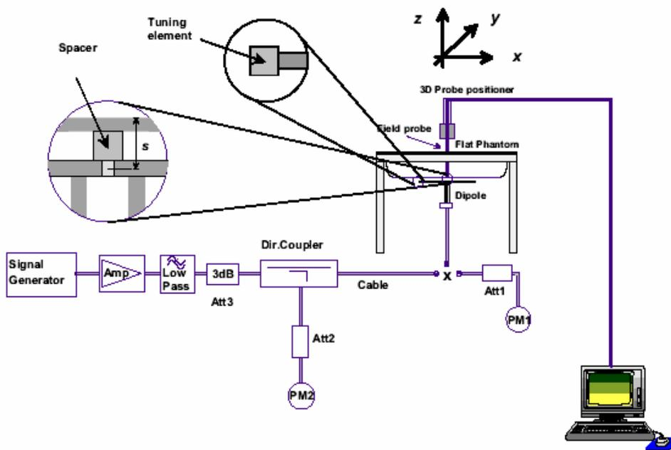
System Performance Check Measurement Setup (IEEE Standard 1528-2003)
