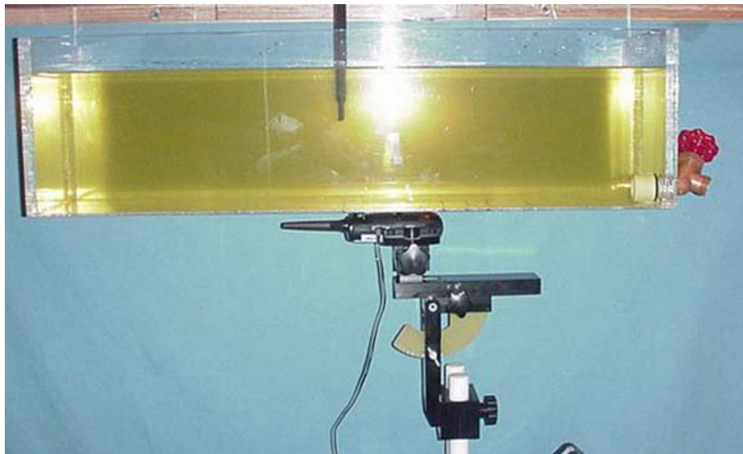
Body-Worn SAR Test Setup Configuration
