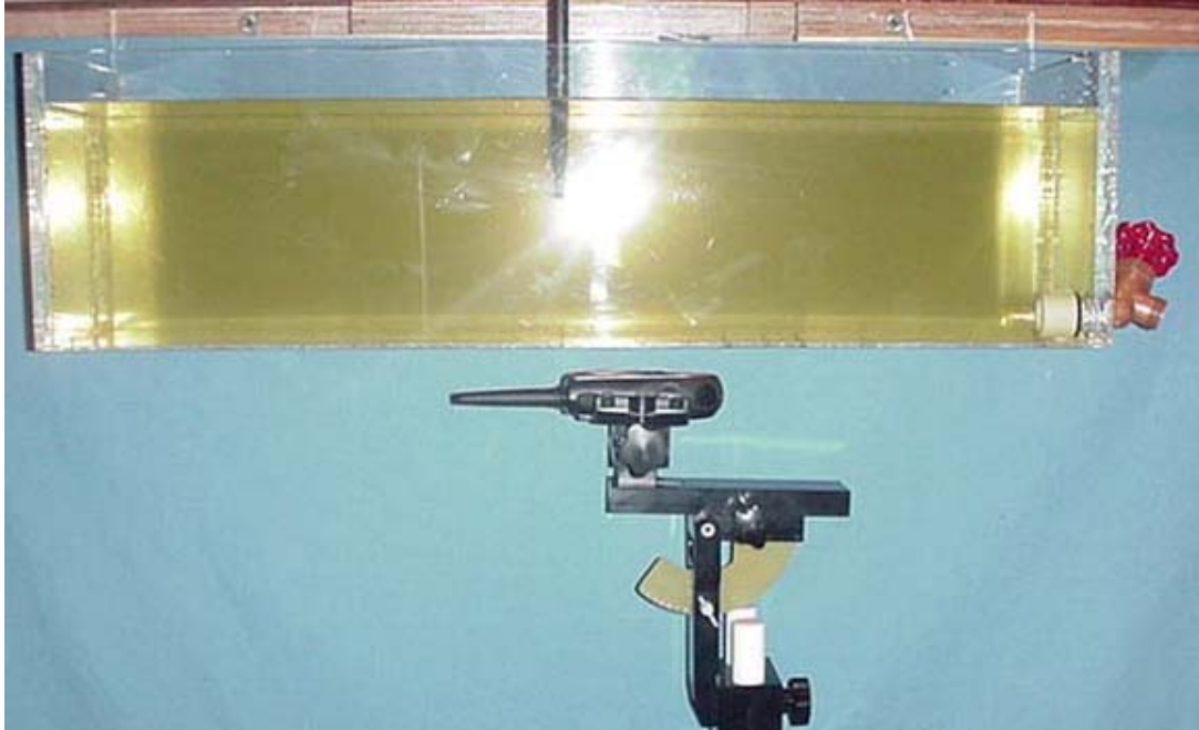
Face-Held SAR Test Setup Configuration
