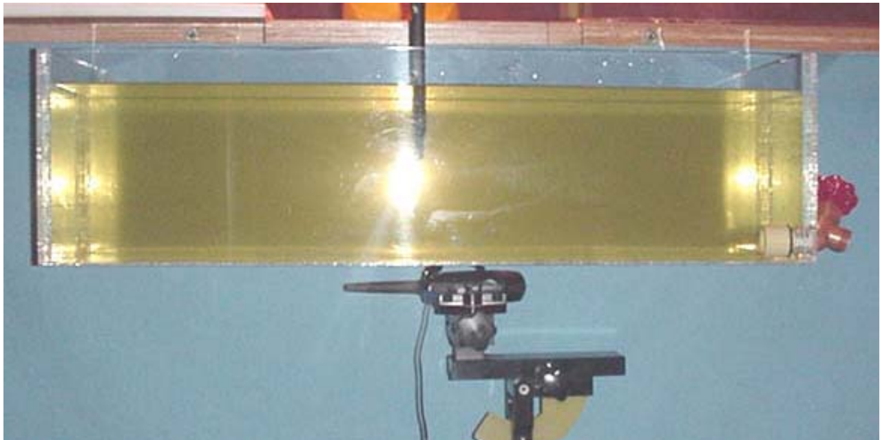
Body-Worn SAR Test Setup Configuration
