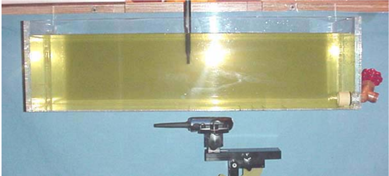
Face-Held SAR Test Setup Configuration
